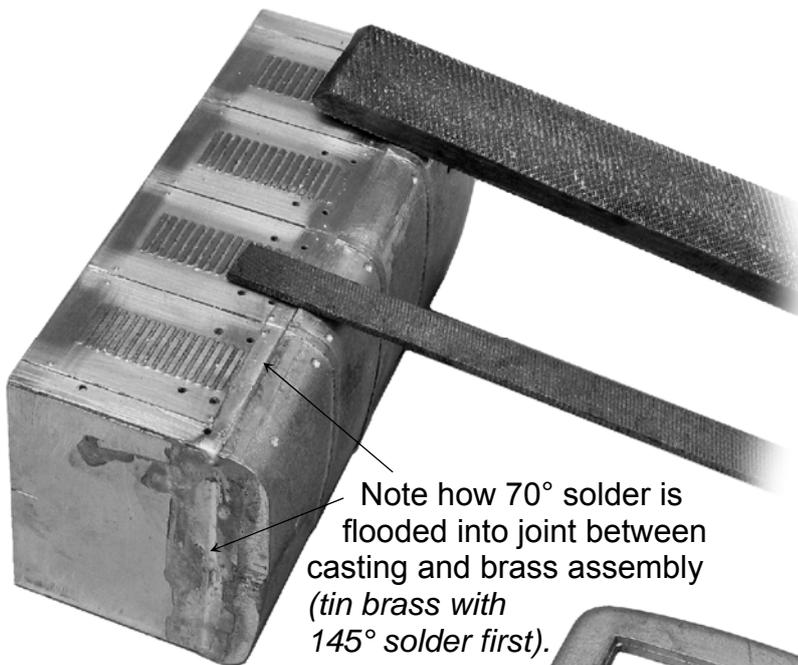
The bonnet top masters included the recommended 2% mould shrinkage allowance. Sods Law says that if you make allowance for it the castings wont shrink (*on the width dimension*). So file bonnet edges down and blend into etched sides. The screw head detail will be lost but it was probably a bit optimistic including it anyway.
