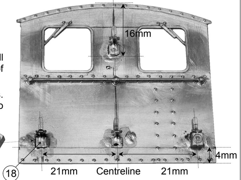
When soldering cab bottom edge to footplate be aware of excessive heat as you don't want the cast lamp boxes falling off.
