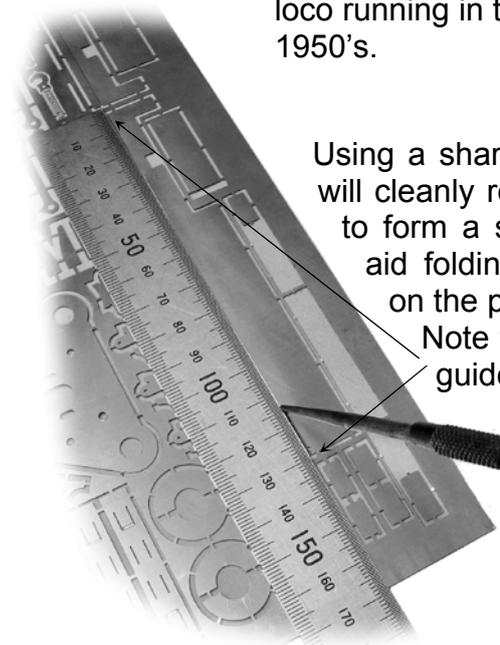
Using a sharp scribe (so that it will cleanly remove a little metal to form a small indentation to aid folding) mark a fold line on the plain underside.
