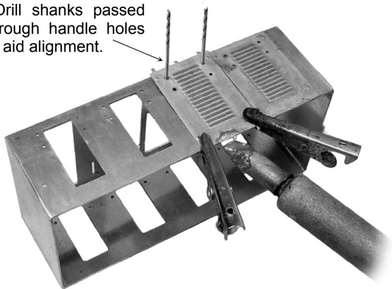
Remove panels from fret and solder into position one at a time. Fit louvered panels first then the small end panels.
