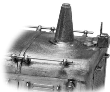
I recommend drilling Ø1.4mm holes & fitting step hand hold (grabhandle) pillars first.
