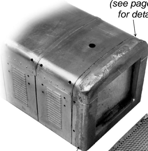
Casting/ low melt solder filed back and then blended into brass bonnet sides by scraping with curved No10 scalpel blade & burnishing with fibreglass brush.
