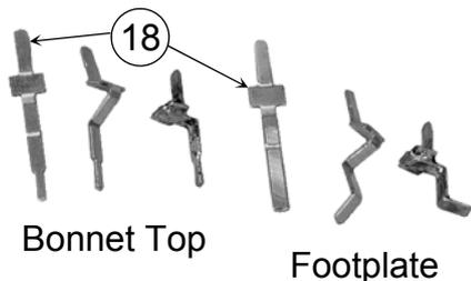
As with the cab back (page 11) the front end was fitted with four fixed electric lamp boxes with lamp Irons incorporated.
