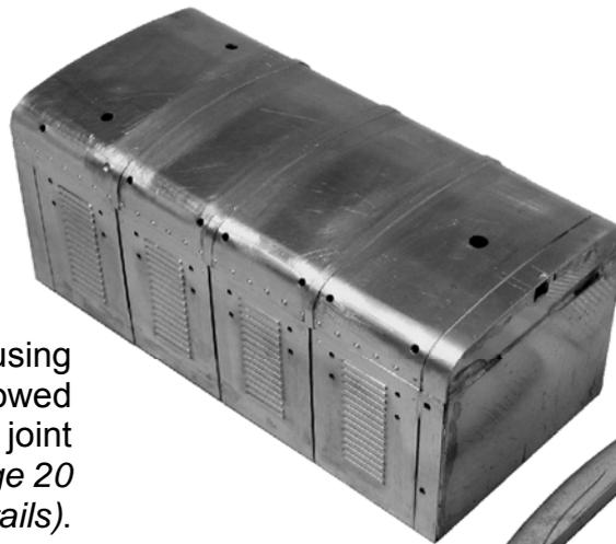
Nose casting is fitted using 70° low melt solder flowed generously into joint (see page 20 for details).
