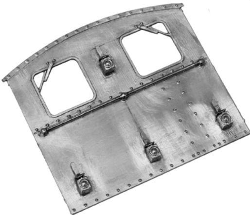
Drewry locos intended for operation over main lines tended to have four fixed electric lamp boxes with lamp irons incorporated. Individual electric lamps could be illuminated or traditional oil lamps or discs carried to display appropriate headcodes.
