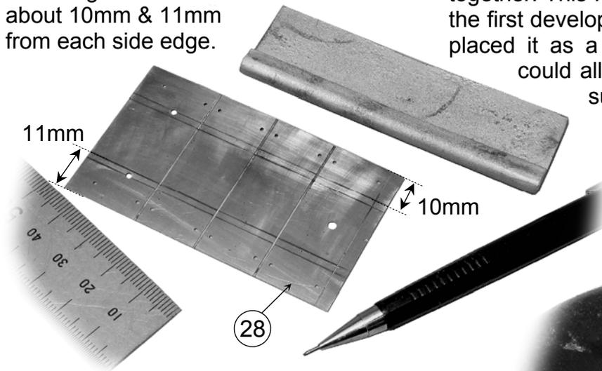
For this sort of job a simple forming bar that the part can be worked over is often fabricated by crudely soldering brass rod & flat together. This I did & used it to form the bonnet for the first development model. I then thought that if I placed it as a master in one of the moulds we could all have one. I found the white metal superior for working the brass over.
