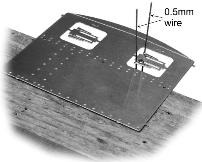
Option 3, Again fit wire tails with wipers retained within window. Then remove and separate into individual wiper arms, bending a slight set on each arm so the blades will sit down within the window opening. Then after fitting window surrounds etc to cab front/back. Place these, inside face downwards, onto a heat proof work block. Positioned overhanging the edge so that the window opening is blocked but the wire tails of the wipers will pass through the above window mounting holes.
