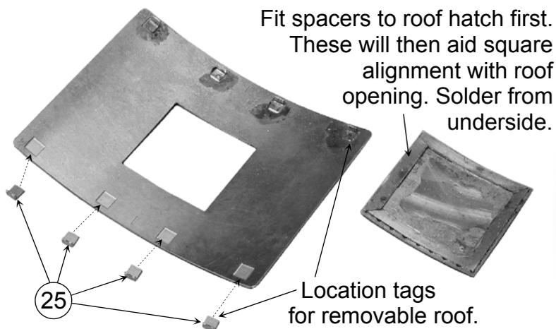
Fit spacers to roof hatch first. These will then aid square alignment with roof opening. Solder from underside.
