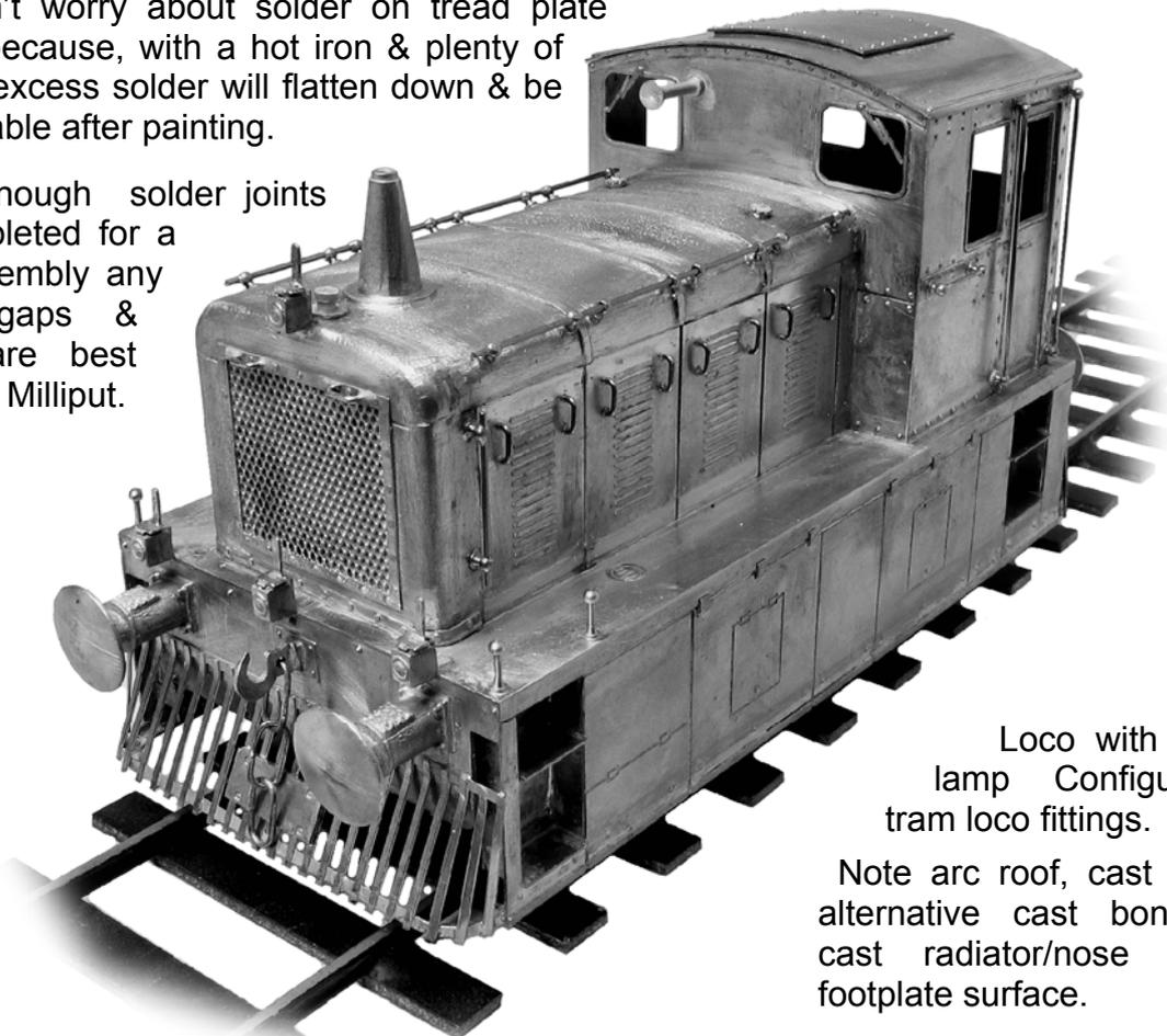
Loco with main line lamp Configuration & tram loco fittings.
