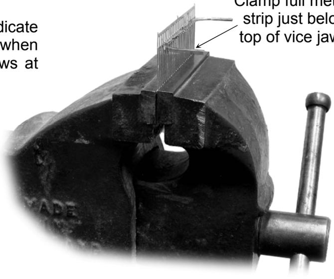
Push steadily forwards, keeping ends of L section parallel to top of vice, until triangles align with Jaws (8mm).
