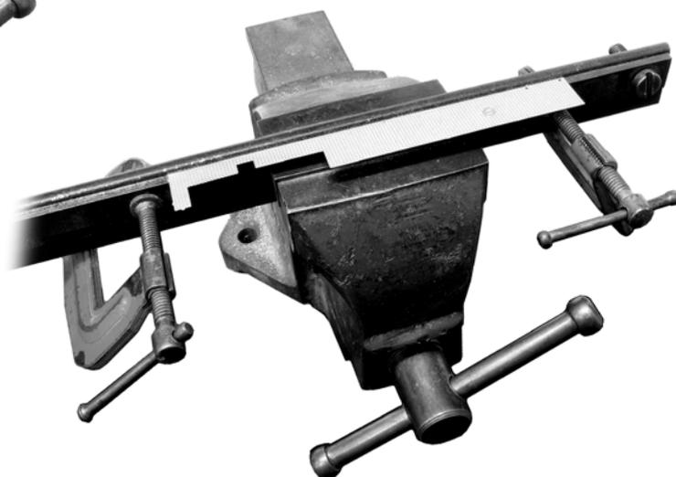
First pre tin the underside (*plain surface*) of all the overlays. Then locate overlay valance over main footplate valance as tight as possible. Note hand gently pressing the footplate edge down onto the work block as finger ends press overlay onto footplate surface using strip of wood (*protection from heat*).
