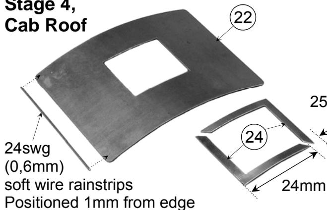
For apex roof, scribe lines on underside of components, note etched centreline marks. Clamp in vice jaws and form slight fold to match cab front/back top edge
