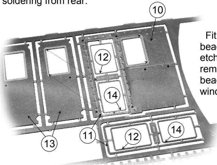
Fit cab side window beading. The half etch rebate should remain visible inside the beadings to represent the windowglass frames.
