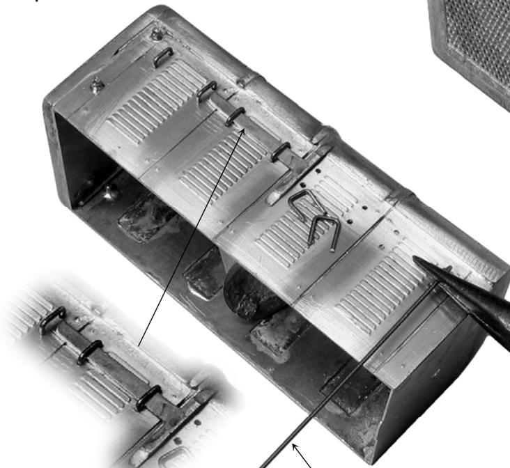
Form access panel handles to be a snug fit into holes so they will retain position when soldered from inside.
