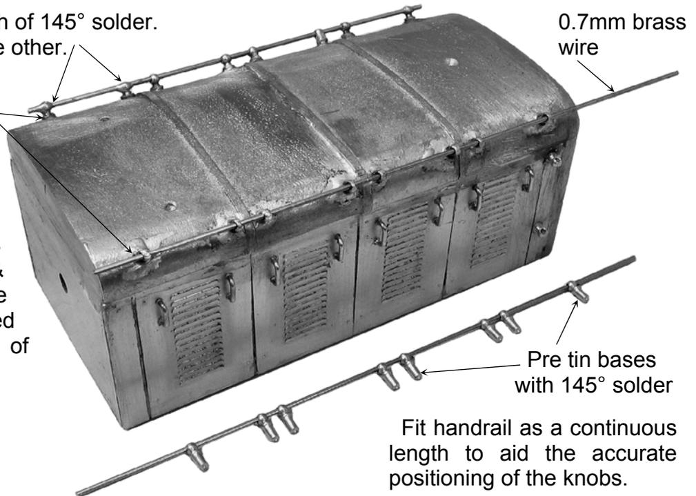
Fit handrail as a continuous length to aid the accurate positioning of the knobs.
