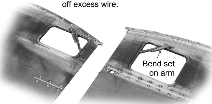
Clean up and dress inside face of window opening so that when, after painting, the glazing is glued into position it will lay flat.
