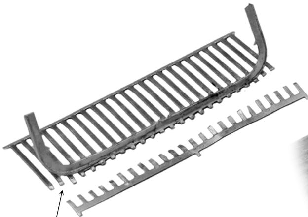
Don't worry about bars being over length and ragged. Cleaning up and levelling of the cow catcher will be done using a flat file after soldering solid between side skirts.
