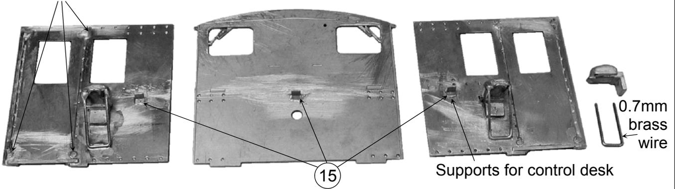
First position seat by eye to just cover etched bolt head embossing holes then check position using driver
