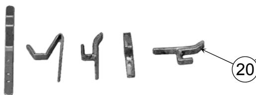
Brackets for stowing the shunters uncoupling pole as he rode along on cab steps
