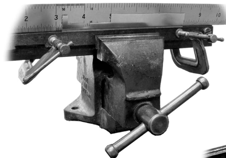
Clamp in folding bars so that scribed line is slightly above (*fully visible*) the top edge of the front bar. A steel rule is used to evenly distribute the folding force as pressure is applied to the back of the rule with finger ends positioned as low as possible (*fingertips touching back bar*).
