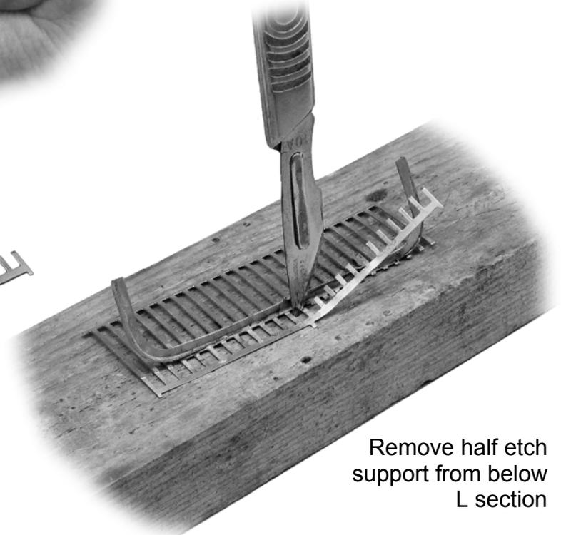
Remove half etch support from below L section
