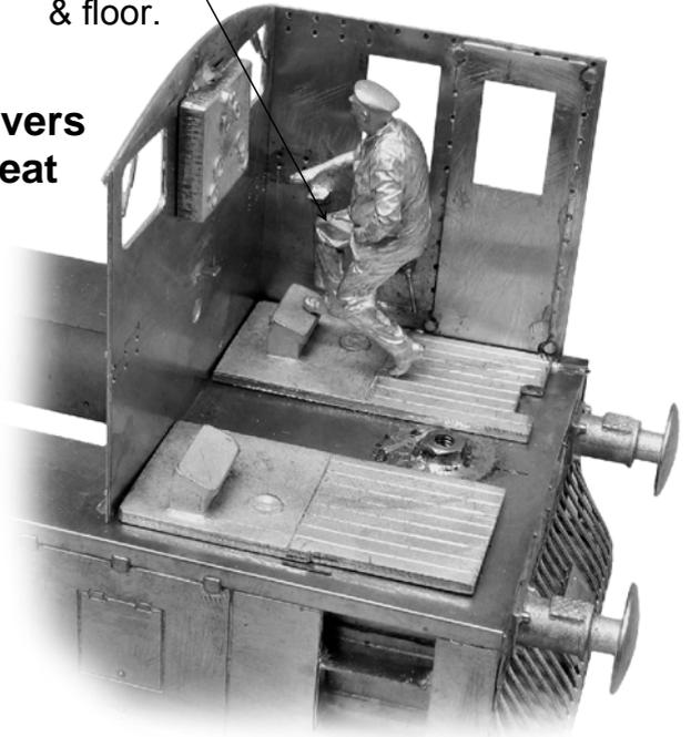
Drill location dimples into seat underside for 0.7mm brass wire
