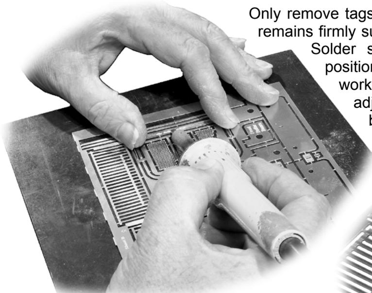
Note half etch (support to be trimmed off latter) uppermost on T10.
