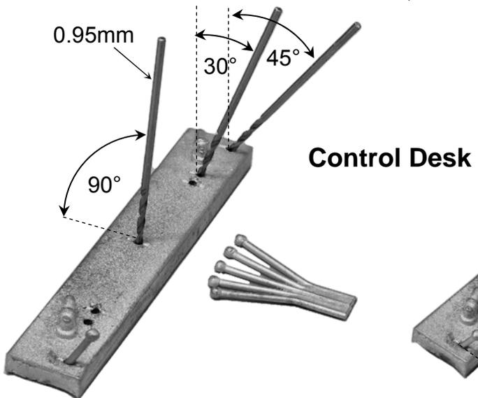
Control knobs should be a positive, but not tight fit, into holes and set (solder on underside) to project about 4mm from desk. so that drivers hand will rest against them.
