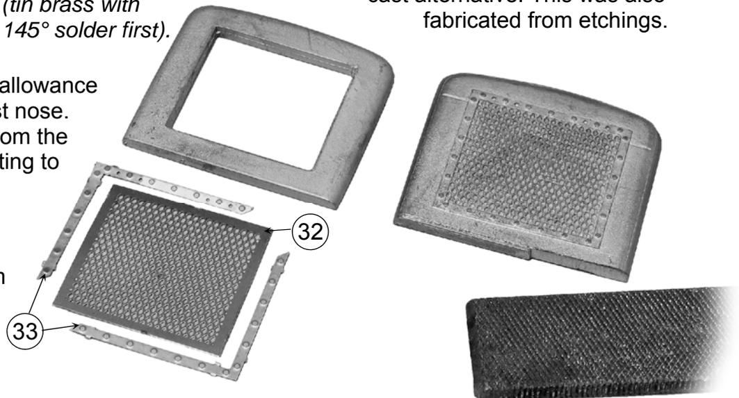
Castings filed back and then blended into brass bonnet sides by scraping with curved No10 scalpel blade & burnishing with fibreglass brush.
