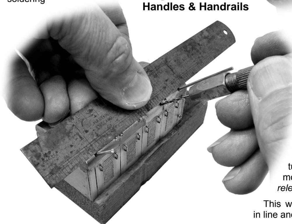
Drill Ø1.5mm holes for outer handrail knobs.
