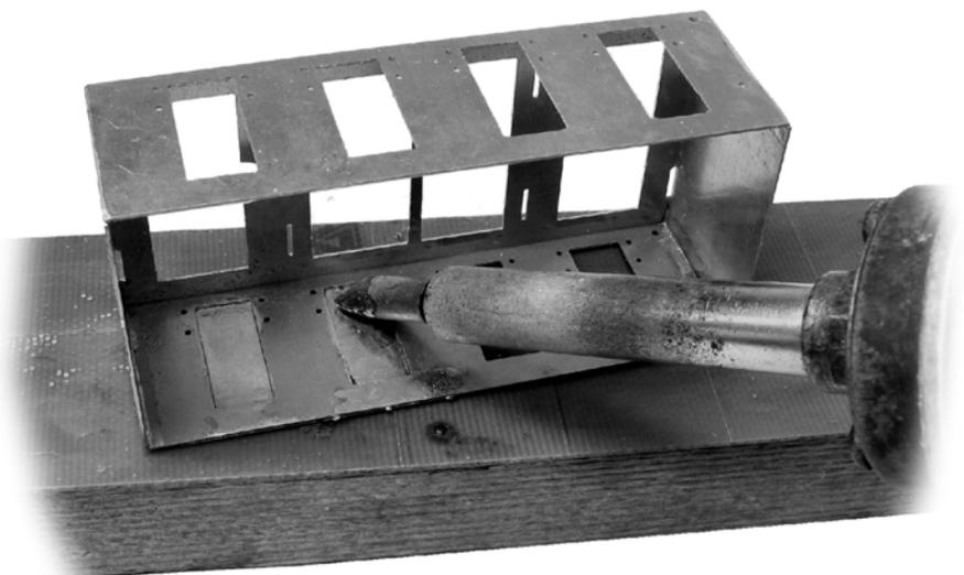
When all side panels are fixed clean off any surface solder from outside faces and clean up louvers (*fibreglass & brass wire brushes*). Then try in position on footplate.
