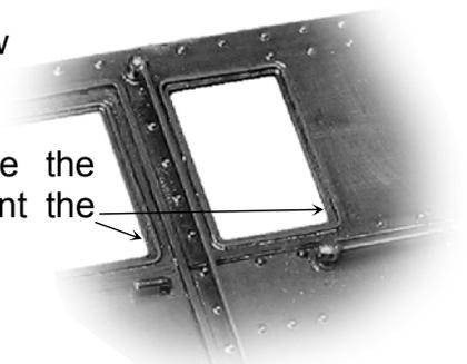
Clean off excess solder & then remove cab sides from fret.
