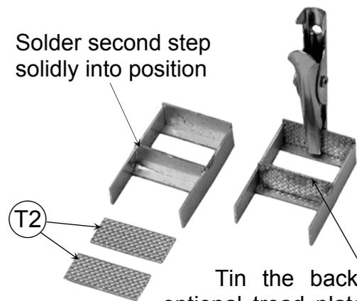
Tin the backs of the optional tread plates before removing from etch. Dress with file to achieve easy fit and solder in position using plenty of flux and application of iron bit to step edge.
