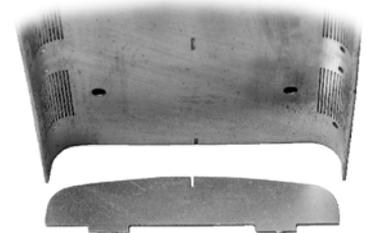
Then form centre curve by gently working with fingers and thumbs over an off cut of copper water pipe. Roll pipe with finger ends as forming pressure is applied by thumbs.
