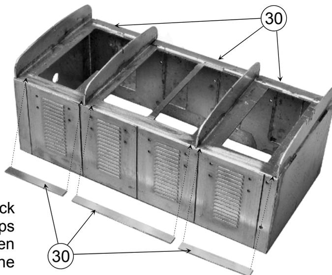
Fit strips flush with or better still just set back from ends of support ribs. These strips provide a useful backing to the gap between the side edges of the bonnet top and the louvered side panels.
