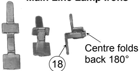
Form up lamp irons and reinforce all folds with 60/40 solder. Tin front & back of square plate with 145° solder.
