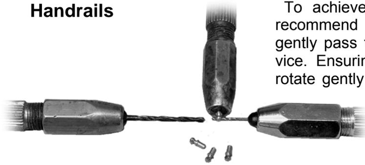
To achieve best results from the handrail knobs I recommend holding base by locking in pin vice. Then gently pass through a 0.75mm drill held in second pin vice. Ensuring that the two pin vices are at 90° and rotate gently and this will correct any misalignment of the cross drilled hole.
