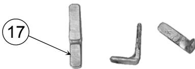
Form up lamp irons and reinforce fold with 60/40 solder. Tin underside of base with 145° solder.
