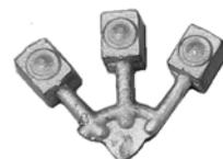
Fit cast lamp boxes using low melt (70°) solder. I was surprised to find this was a fairly easy operation.
