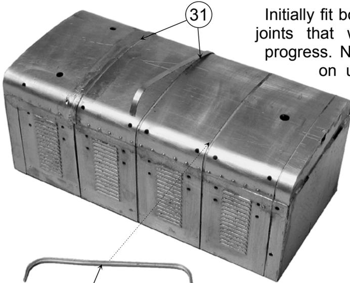
Initially fit bonnet top using a number of small tack solder joints that will allow adjustment, if required, as you progress. Note corresponding etched centre line marks on underside that correspond with support ribs.
