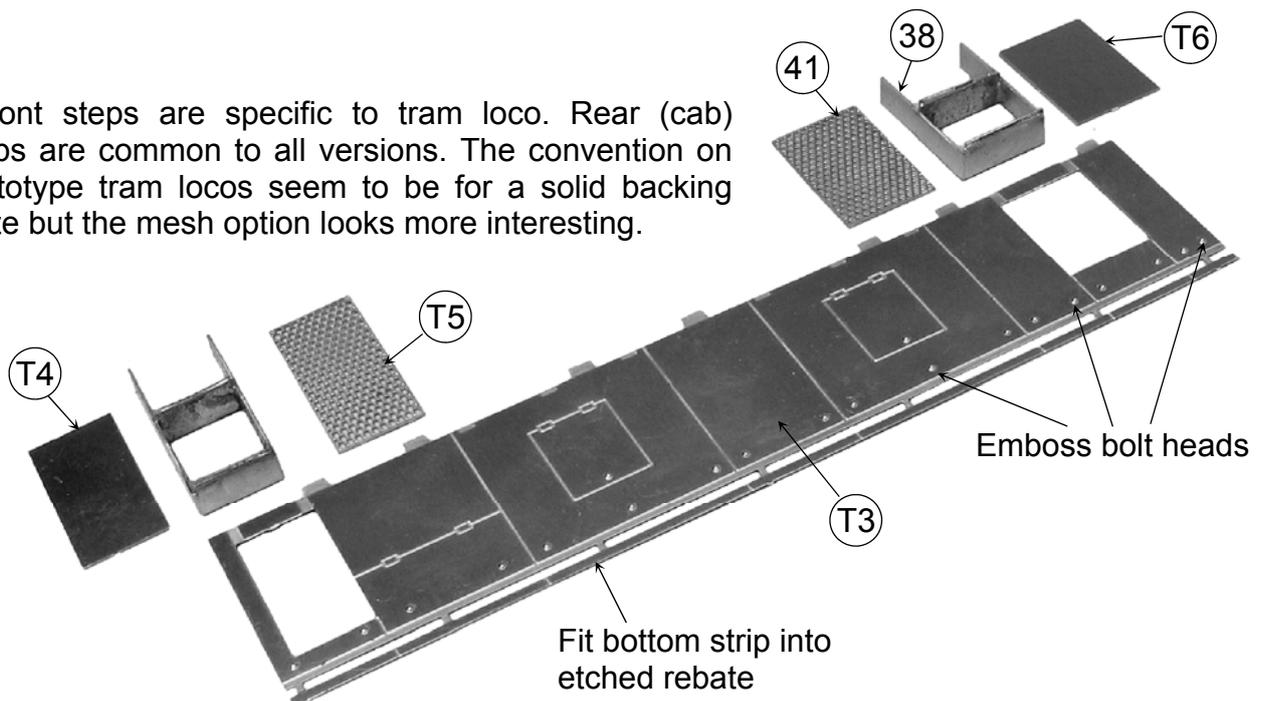
When backing plates are solidly fixed snip out top strengtheners from cut outs.
