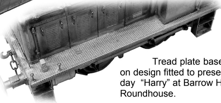
Tread plate based on design fitted to present day "Harry" at Barrow Hill Roundhouse.
