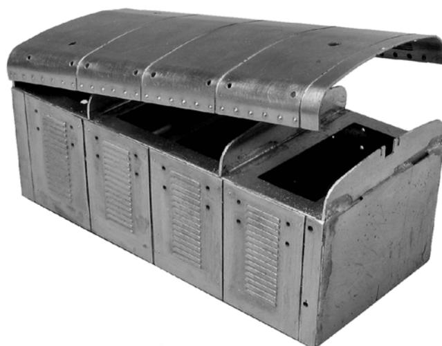
The support ribs are there to work for you by providing a framework that will achieve a level bonnet top with consistent corners & top radius. If you are having to force it down over them, then they are working against you, so don't be afraid to slightly dress and re-profile ends so that bonnet top is a snug fit. With sides sitting down just above the louvered panels with a consistent gap (about 0.5mm).
