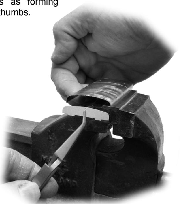
Side bends are now excessively tight so clamp sides (bottom flat 1mm) in vice jaws & ease up slightly to match support rib profile.
