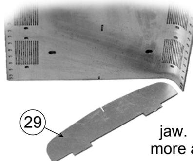
Offer up a support rib to check start of bend position. If low clamp & flatten edge slightly in vice jaw. If high form over more at edge.
