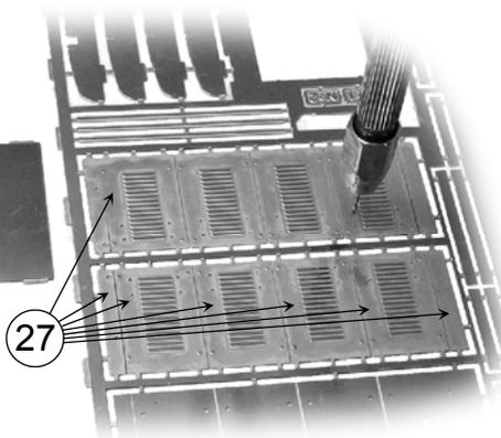
With bonnet side sheets retained within fret drill through lifting handle holes 0.75mm to ensure all have the same clearance diameter.
